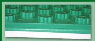
Make sure sub grade material is + or - 1/4" of level to start. To lay the boards correctly, start at the far left-hand corner and work systematically across the floor as numbered on the sample. The only cut off is for the partition wall. The Crete-Heat  $^{TM}$  Panel modular board system by Crete-Heat, LLC form a continuous thermal insulation, and vapor barrier with tube fasteners all in one simplified step.
