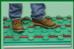
The Crete-Heat™ Insulated Floor Panel System is an easily assembled modular board insulation, vapor barrier and radiant tube holding grid. It allows for simplified installation of hydronic radiant floor heating systems in basements, garages, main floor slab on grade and above grade installations where concrete or gypcrete is normally used.
