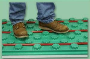
The Crete-Heat<sup>™</sup>Insulated Floor Panel System is an easily assembled modular board insulation, vapor barrier and radiant tube holding grid. It allows for simplified installation of hydronic radiant floor heating systems in basements, garages, main floor slab on grade and above grade installations where concrete or gypcrete is normally used.
