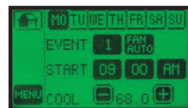
Pre-program up to 4 temperature and fan operation mode changes daily
