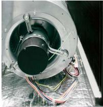
Foil faced insulation in the blower section and fiberglass insulation in the compressor section
